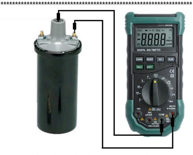
SECONDARY TEST 200K OHM SCALE
