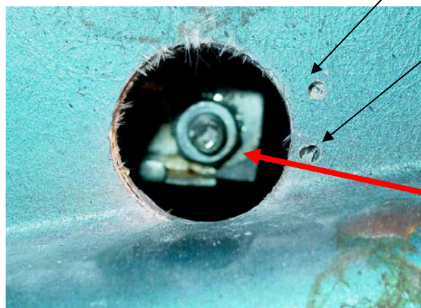
Sash stud and nut at front of window
