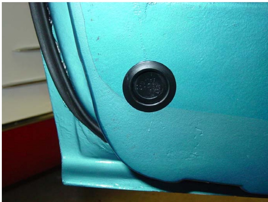
Used clutch hole plugs that I got from LIC to close the holes
